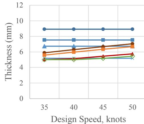
Minimum Bottom Plating Thickness @ 0.875L
