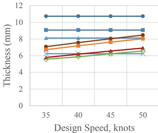
Minimum Bottom Plating Thickness
