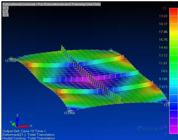
Figure 10: The computational result of total deformation. [1]
