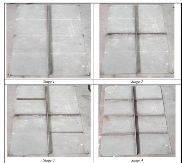
Figure 8: Welding process stages in the case study 5.
