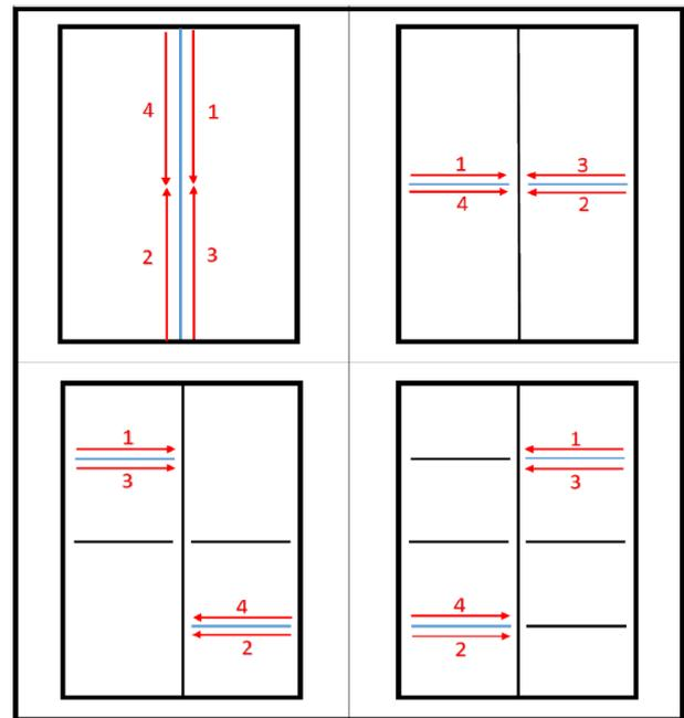
Figure 7: Welding sequence in the case study 5.
