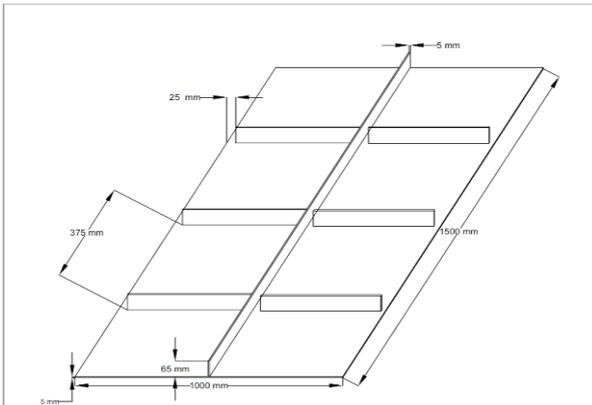
Figure 3: CAD Model with a base plate, one longitudinal flat bar and three transverse flat bars.
