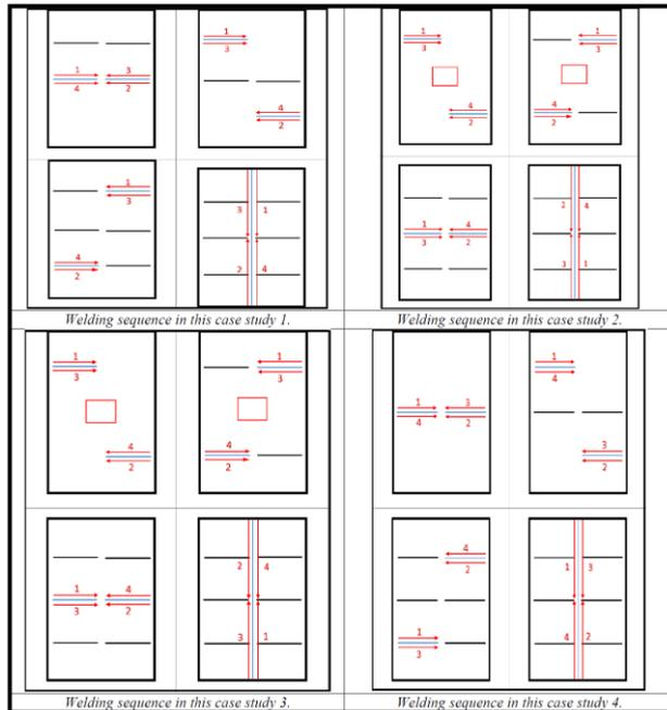
Figure 5: Welding sequences in the case study 1 to 4.
