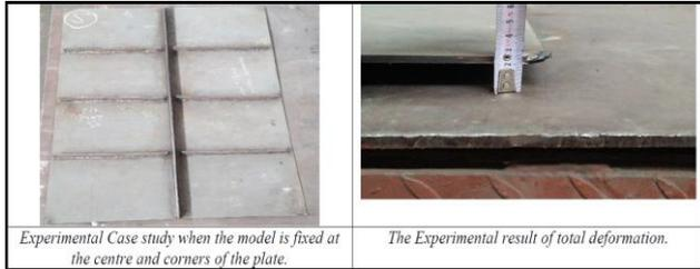
Figure 9: Total welding deformation result for case study 5.
