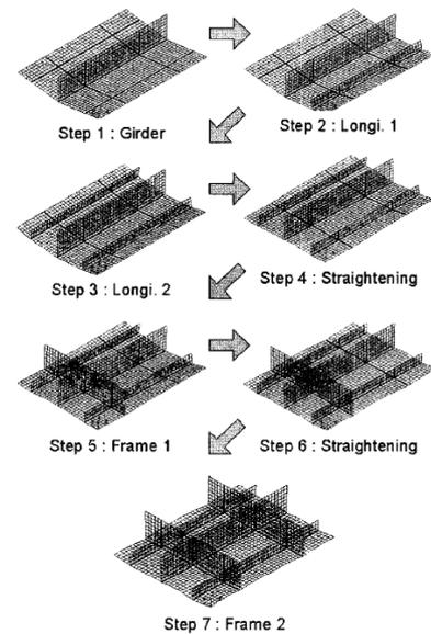
Figure: Welding deformation of each assembly stage
