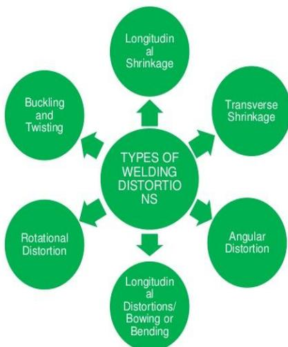
Figure 1: Types of Distortion in welding [2]
