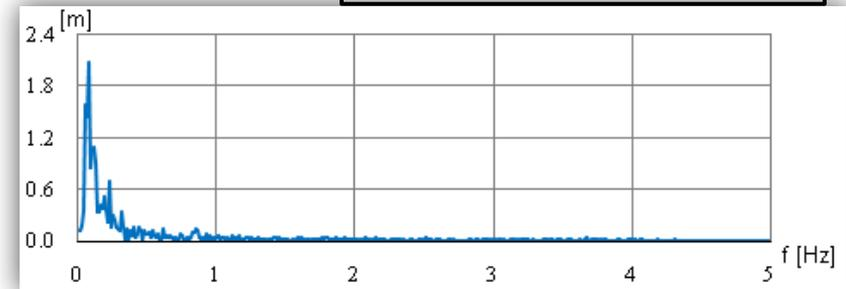
The dynamic bending moment at hydroelastic linear and non-linear analysis, significant wave height  $h_{1/3}=10.65\text{m}$  at  $x/L=0.5$
