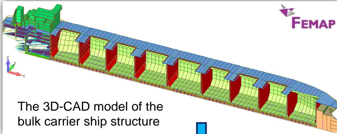
The 3D-CAD model of the bulk carrier ship structure
