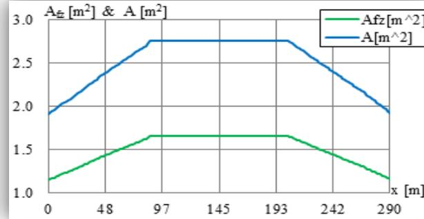
The diagram of the total area and shear area
