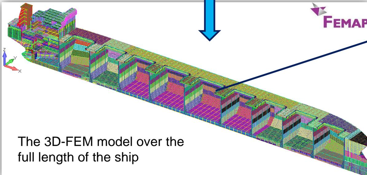
The 3D-FEM model over the full length of the ship
