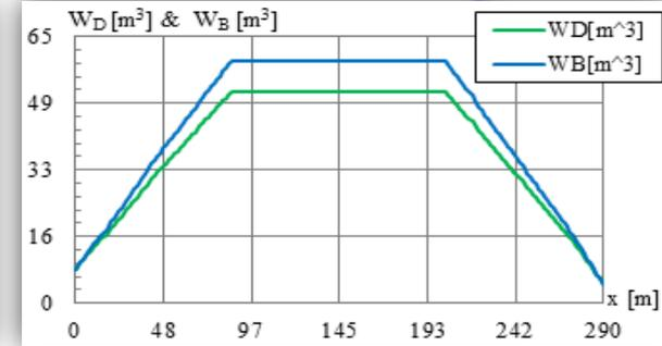
The diagram of the bending resistance modules of the extreme fibre for bottom and for deck
